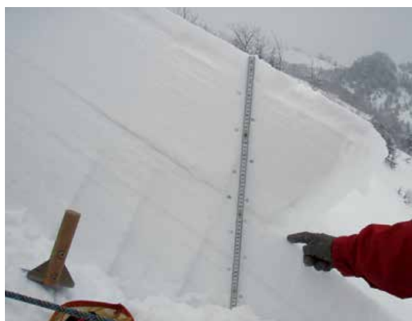
図4 破断面における積雪の鉛直断面写真(左)と断面観測結果(右) Fig. 4 Photograph of the vertical cross section (left) and physical property profiles (right) of the snow cover at the crown surface.
