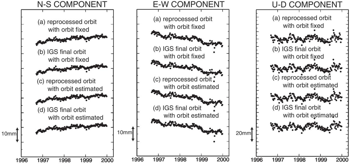
**Fig. 3** Time series of the baseline between 3097 and 3078 sites in the Tokai network. (a) Applying the reprocessed orbit with orbit parameter not estimated. (b) Applying the original final orbit with orbit parameter not estimated. (c) Applying the reprocessed orbit with orbit parameter estimated. (d) Applying the original final orbit with orbit parameter estimated.
