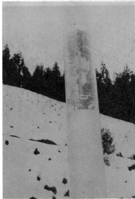
写真-5 積雪深計頭部 Capsule of the snow-cover height meter.
