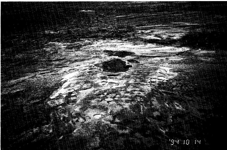
写真17 花咲港東地区埋め立て地の噴砂口 Photo 17 A Series of Sand Boils (Reclaimed Land, Eastern Area, Hanasaki Port)
