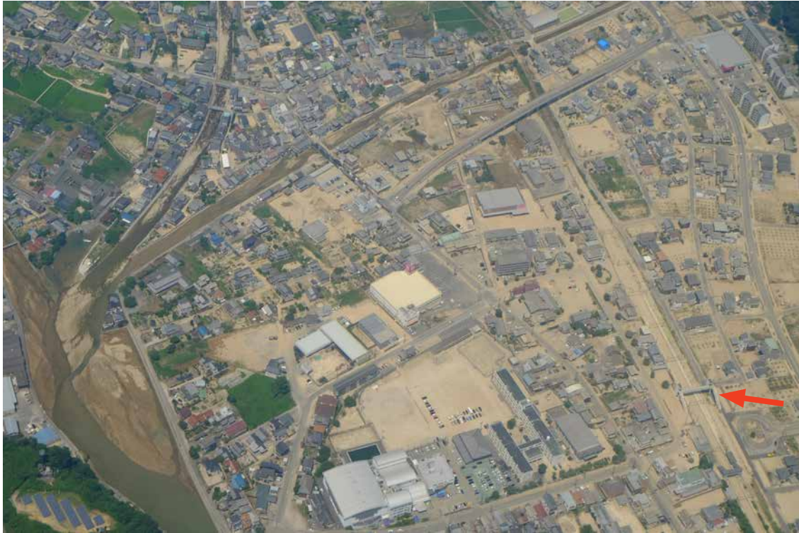
口絵 5 JR呉線安浦駅(矢印)周辺の浸水に伴う土砂の堆積状況(撮影:2018年7月25日,広島県呉市安浦町中央) Fig. 5 Sediment accumulation due to inundation around Yasuura Station on JR Kure Line, indicated by the red arrow (July 25, 2018: Chuo, Yasuura-cho, Kure City, Hiroshima Prefecture).
