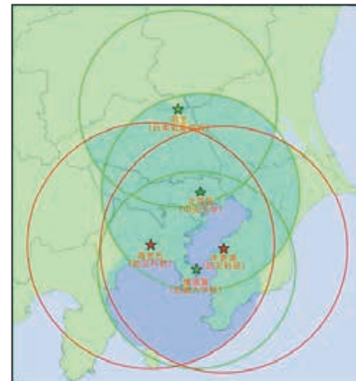
図1 X-NETのレーダ設置位置と観測範囲 Fig. 1 Location of X-NET Radar (asterisk) and its observation area (light green shading).
