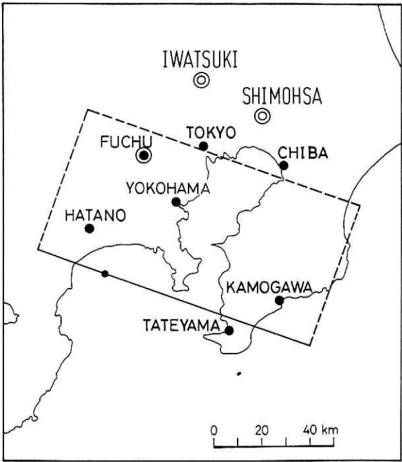
Fig. 2 Projection of the assumed fault plane upon the ground surface, and positions of Tokyo, Yokohama, Hatano, Fuchu, Chiba, Kamogawa, and Tateyama where the strong ground motions are synthesized. Double circles are the three Deep Borehole Observatories of Iwatsuki, Shimohsa, and Fuchu where down-hole measurements were carried out for precise estimation of the sedimentary structure.
