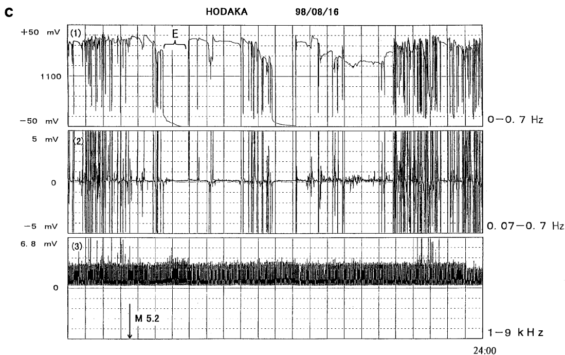
Fig. 15c The monitoring records on 16 August, 1998 when the largest earthquake with magnitude of 5.2 occurred. Transient SP anomalies consisted of a typical type of fluctuation seen as “high” frequency pulse signals of negative polarity and variable duration, from several seconds to tens of minutes. The sharp drop at the initial stage, followed by gradual decrease to saturation, and final sharp recovery is well exemplified in (1). It should be noted that these were accompanied by only minor anomalous signals in the ELF/VLF channels (3) in comparison with other channels. Digitized data for 15 August could not be recovered because of modem trouble at the time of the severe shock induced by the largest earthquake. The paper monitoring chart, however, shows that a very large increase in electric field anomalies occurred about 10 hours before the earthquake. The anomaly is several times larger compared with those on previous days, even causing a recording malfunction due to paper breakage induced by large fluid ink drainage, which indicates rapid and large signal occurrence.
