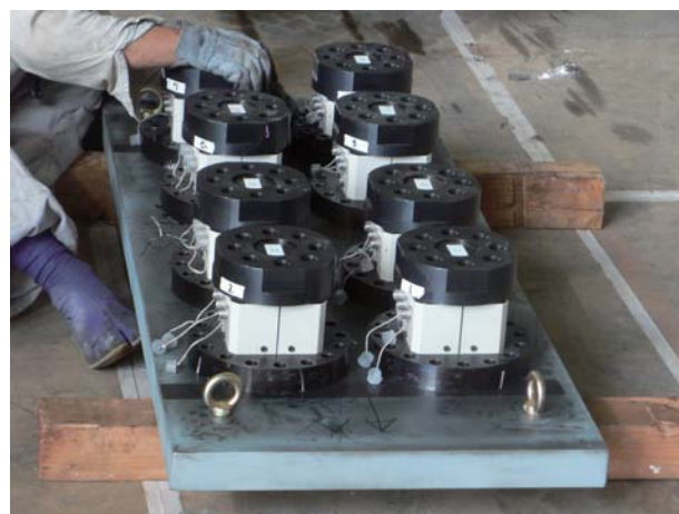
写真 24 端部架台上三分力計 (8 個設置) Photo 24 Loadcell for movable bearings.
