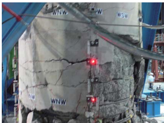
写真 52 C1-5(3)2 回目加振後北面 Photo 52 Damage on north face after C1-5(3)-2 excitation.
