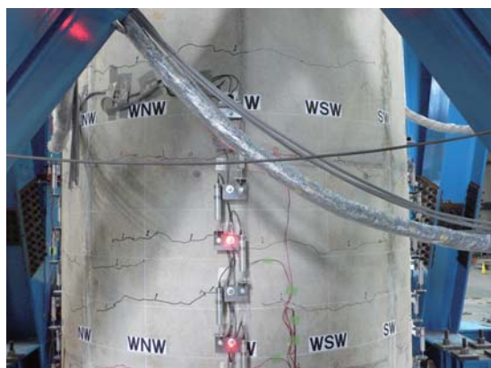
写真 30 C1-5(1)1 回目加振後北面(計測室側) Photo 30 Damage on north face after C1-5(1)-1 excitation.
