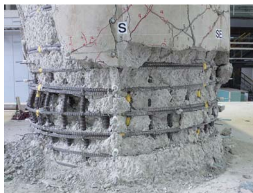
写真 60 C1-5(1)(2)(3)実験終了後南面 Photo 60 Damage on south face after C1-5(1)(2)(3) excitations.
