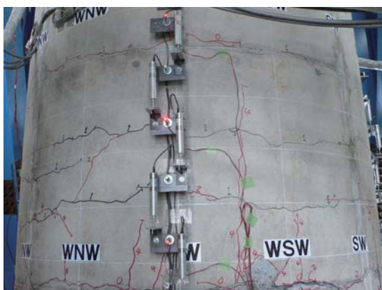
写真 38 C1-5(2)加振後北面(計測室側) Photo 38 Damage on north face after C1-5(2) excitation.
