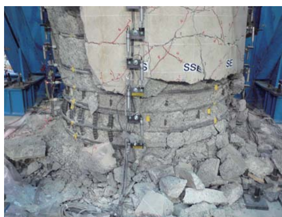
写真 54 C1-5(3)2 回目加振後南面 Photo 54 Damage on south face after C1-5(3)-2 excitation.
