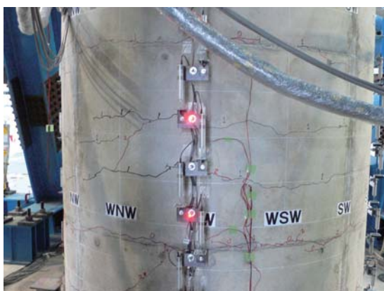
写真 34 C1-5(1)2 回目加振後北面(計測室側) Photo 34 Damage on north face after C1-5(1)-2 excitation.
