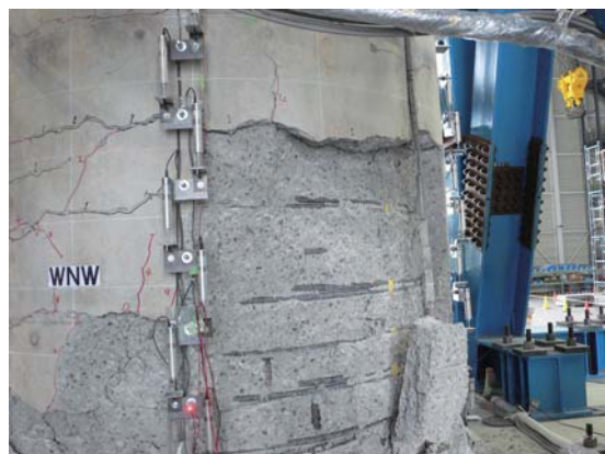
写真 48 C1-5(3)1 回目加振後北面 Photo 48 Damage on north face after C1-5(3)-1 excitation.
