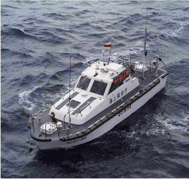
Fig. 4 The manned/unmanned survey boat Manbo II . It is usually mounted on a large survey ship and used in places the mother ship cannot enter.
