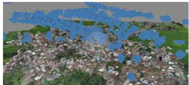
**Fig.7.2** 3D digital surface models of buildings using PhotoScan™ for Sankhu. Blue rectangles show camera positions and orientations determined by PhotoScan™.
