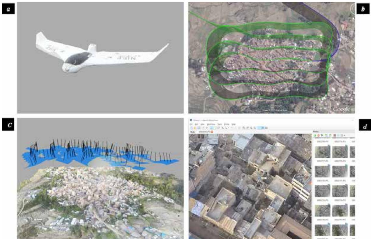
**Fig. 7.3** Building damage survey using compact UAV over Khokana.
