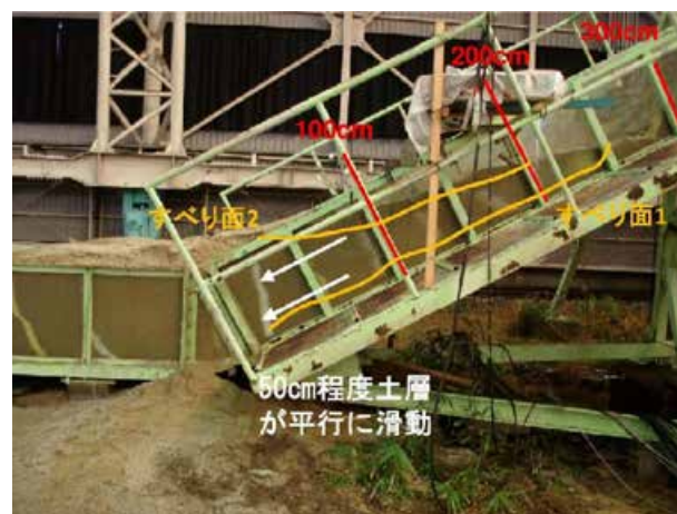
写真1 崩壊後の模型斜面(側面) Photo 1 Lateral view of the failed slope.
