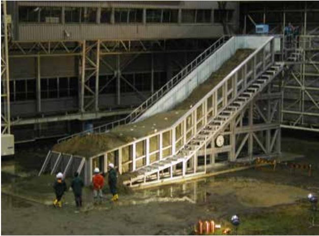
図2 実大規模の斜面崩壊実験 Fig. 2 Full-scale landslide experiment.
