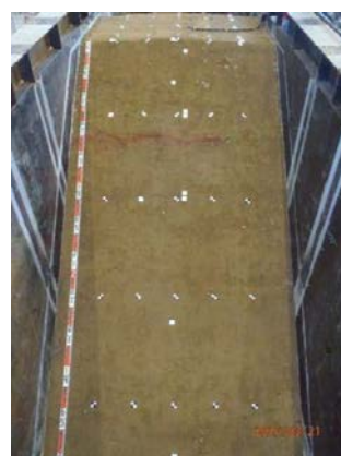
写真 23 前刃金下流法面クラック発生状況 Photo 23 Distribution of cracks on the slope surface of downstream in the case of sloping core zone.
