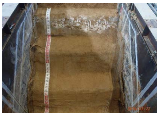
写真 31 シート側段切り部石灰到達状況 Photo 31 Confirmation of the lime filled into the cracks along the GCL on the bench-cut surface.
