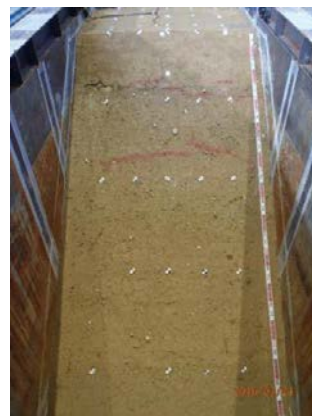
写真 21 前刃金上流法面クラック発生状況 Photo 21 Cracks occurred in the slope surface of upstream in the case of sloping core zone.
