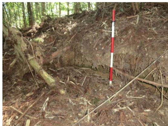
写真3 地すべり地形Aの滑落崖 Photo 3 Head scarp of landslide configuration A.
