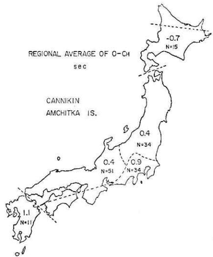
Fig. 17. Regional average of the traveltime residuals for the nuclear explosion Cannikin. Dotted lines are boundaries of the regions. *N* is the number of the observations used in averaging (after Hamada, 1973).
