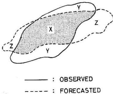
**Fig. 2** Conceptual illustration of overlapping of two echoes. The area inside the solid line shows the observed echo and the area of broken line shows the forecasted echo. Part X is the "overlapped" area, parts Y are "observed but not forecasted", and the parts Z are "forecasted but not observed".
