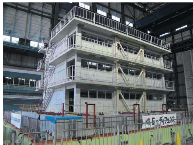
3層試験体・耐震補強有り 3-story specimen with seismic retrofitting
