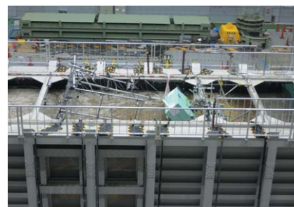
実験後海側へ1m以上動いたケーソン護岸と基礎構造物 The caisson revetment and pile foundation structure moved seaward by more than 1 m
