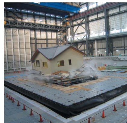
震災復旧・免震建物実験 Test on rehabilitated and seismic isolated house
