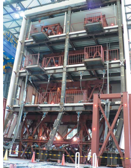
4層建物の崩壊状況 4-story full-scale steel building following test
