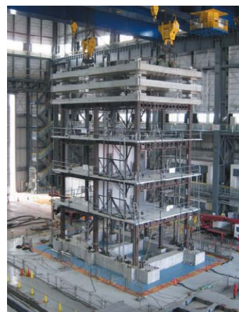
試験体全景 Specimen modeled High-Rise Buildings
