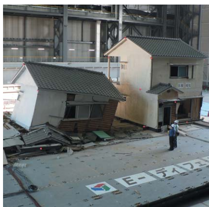
移築補強・無補強建物実験 Test on reinforced and non-reinforced houses
