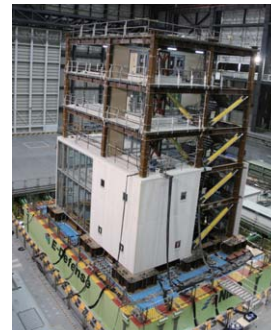
制振試験体 Specimen with damping systems
