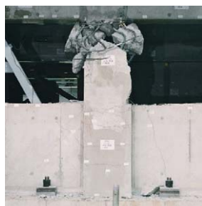
1層柱のせん断破壊 (2005年度) Shear failure of 1st-story column
