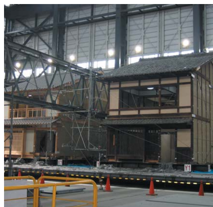
移築・新築伝統建物実験 Test on relocated and new traditional-style houses
