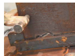
実験後梁端溶接部破断(拡大) Welding break at end of girder after test (enlarged)
